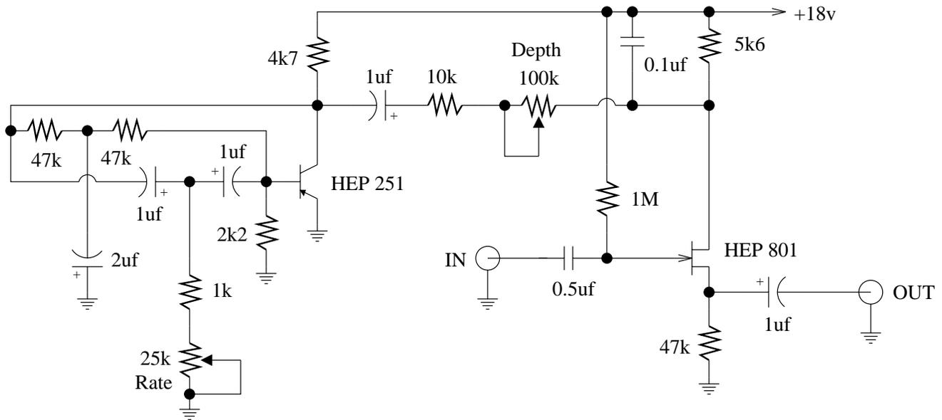
This tremolo circuit is not a "plug and play" ready guitar effect, however it could be converted to one with relative ease. It just needs some buffering on the input and output and perhaps some bypass switching.
