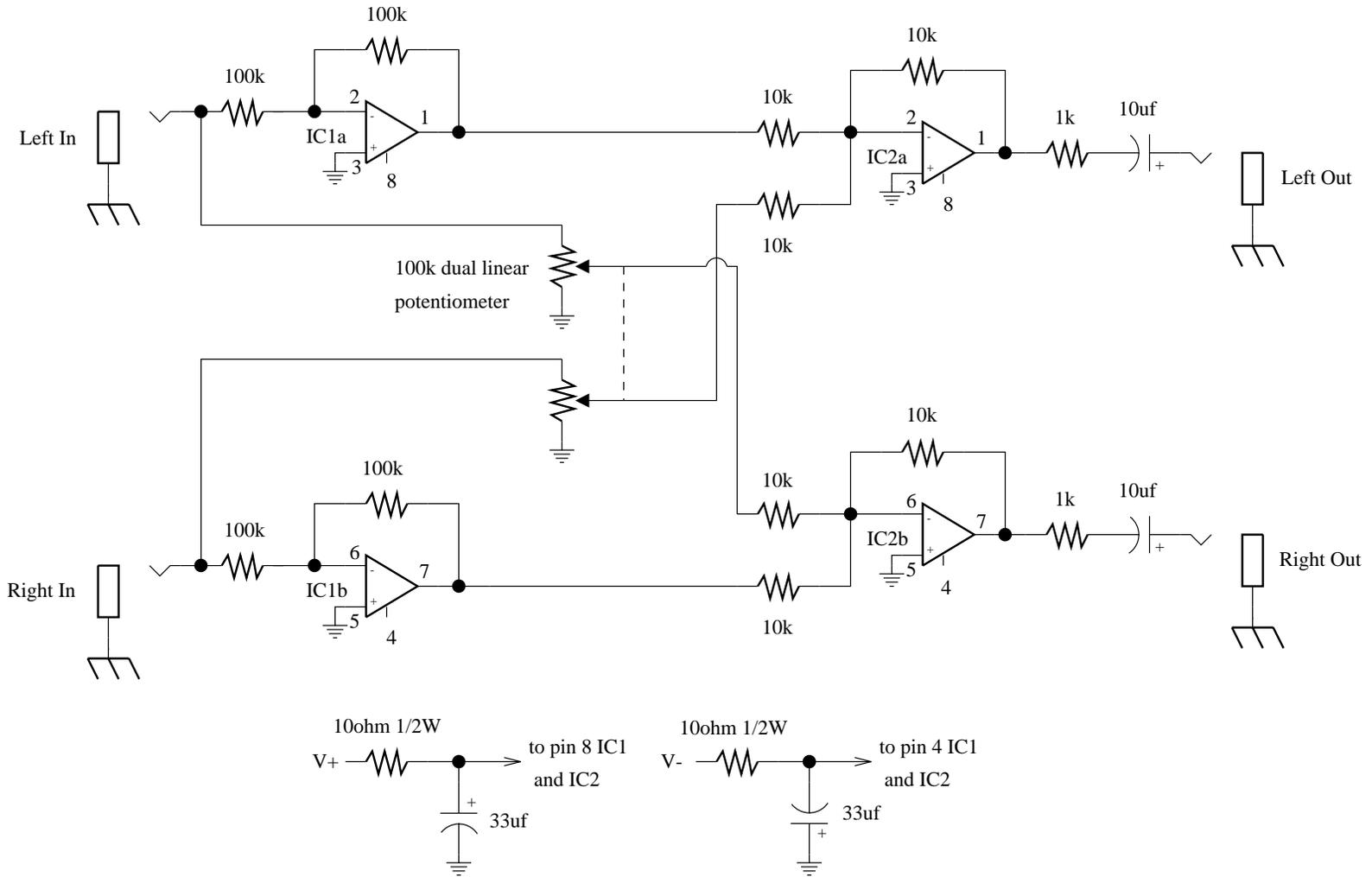
IC1 & IC2 are 5532 Dual Op amps for low noise. All resistors are 1% metal film 1/4W unless otherwise noted. Requires bipolar power supply from 9 to 15 volts.
