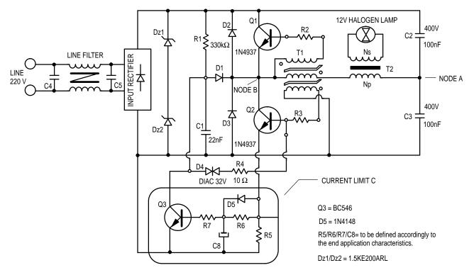
Figure 1. Basic Schematic Diagram for a 12 V Electronic Transformer
