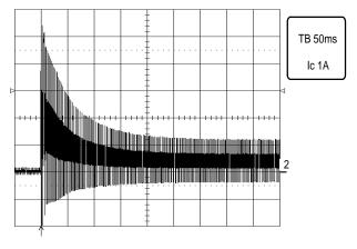
Figure 3. Start Up Collector Current (50 W Transformer), the mains being replaced by a DC power supply V<sub>CC</sub> = 240 V, T<sub>amb</sub> = 23°C.
