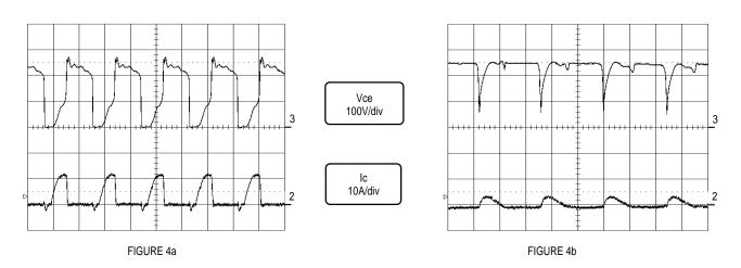
Figure 4. Short Circuit Conditions in a 150 W Converter with  $V_{CC}$  = 240 V.
