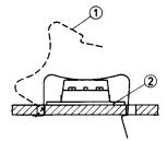
Fig 7. Mounting. (1) spring clip. (2) insulator.
